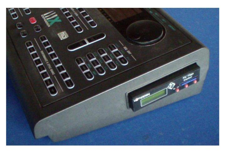
The original floppy of the Generalmusic WX-Expander is an extra small type. There is not enough space for the SD type of the HxC floppy emulator. A solution for this problem is to let project the emulator 11mm over the housing of the WX-Expander. To arrive this solution, two mechanical modifications are to do.
