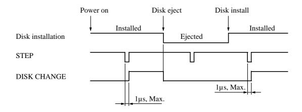
Note: To simplify the timing chart, the DRIVE SELECT signal is assumed always TRUE in the above figure.
