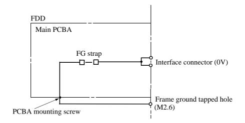
(Fig. 10-1) Frame ground internal connection
