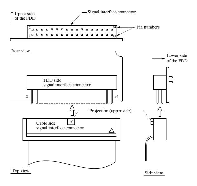
(Fig. 8.1-1) Signal interface connector external view
