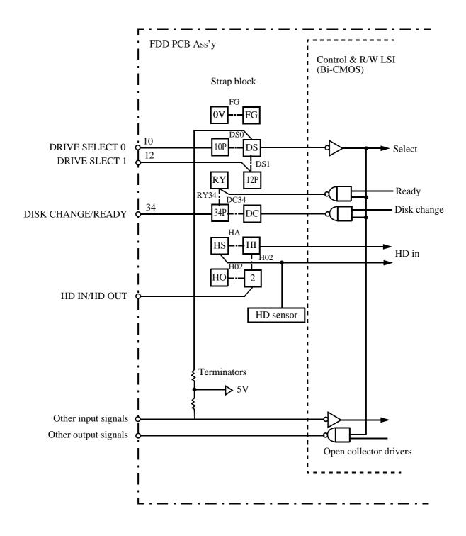
(Fig. 8.2.2-1) FDD signal interface circuit
