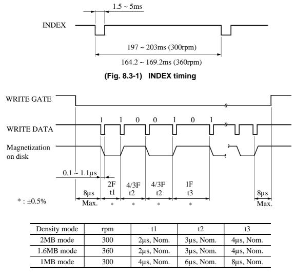
(Fig. 8.3-2) WRITE DATA timing (MFM method)
